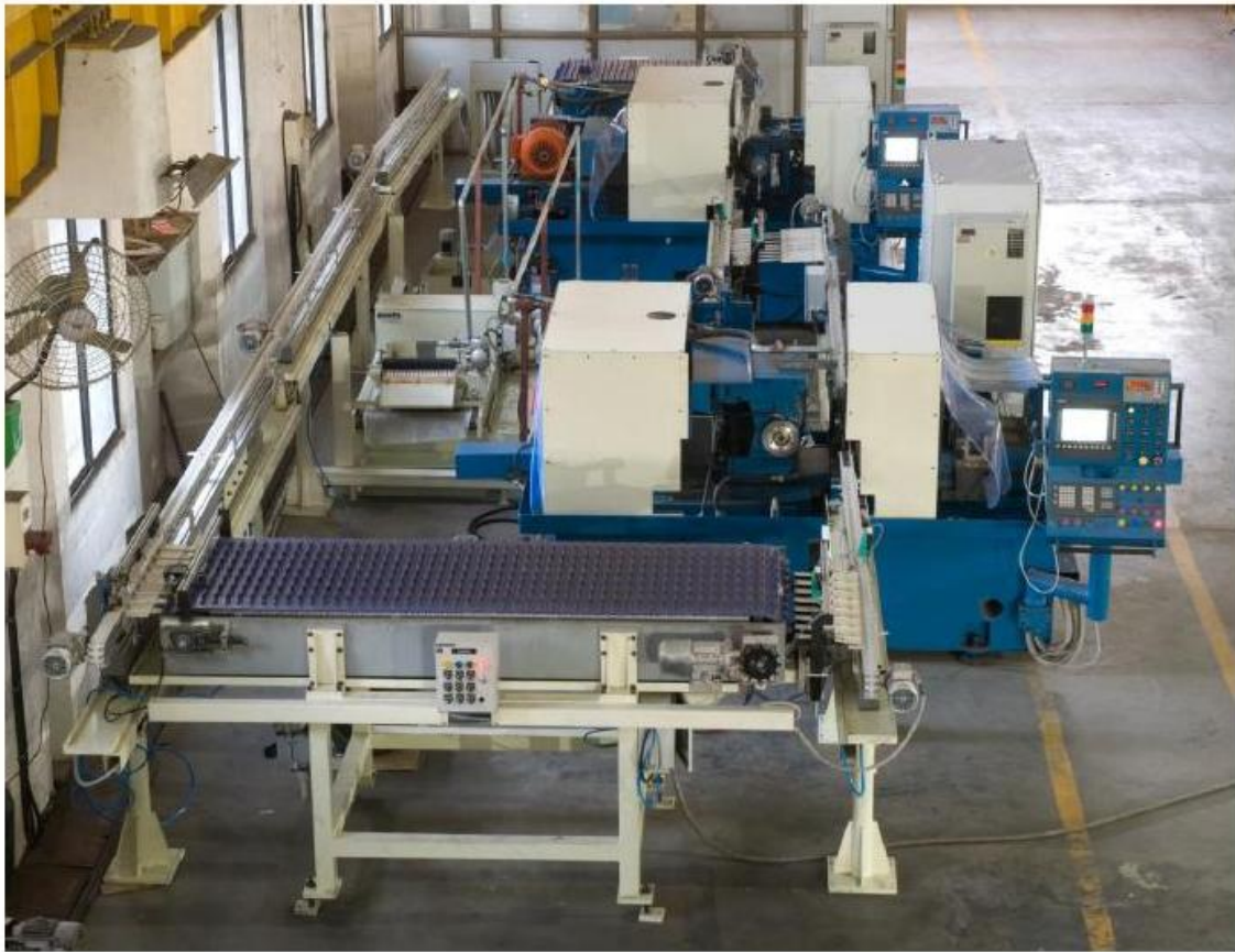
Line of SMT-Bocca CNC Centerless Grinder Model R-50 for Lakshmi Machine Works, Coimbatore
