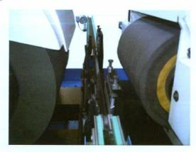
Bocca & Malandrone centerless are completely CNC controlled. As shown in the sketch, the grinding wheel axis named (X2) manages the grinding wheel slide movement toward dressing unit and backward to the blade (the part to be machined), as well the control wheel axis named (X1) manages the control wheel slide movement toward the dressing unit and backward to the blade (the part to be machined).
