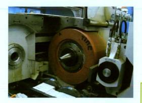
The patented BMS solution permits to change the grinding and regulating wheel rapidly without disassembling the spindle from the machine by means of open-able wheel front support.
