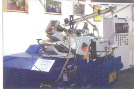
No.2 CNC Groove Grinder for Engine Valves
